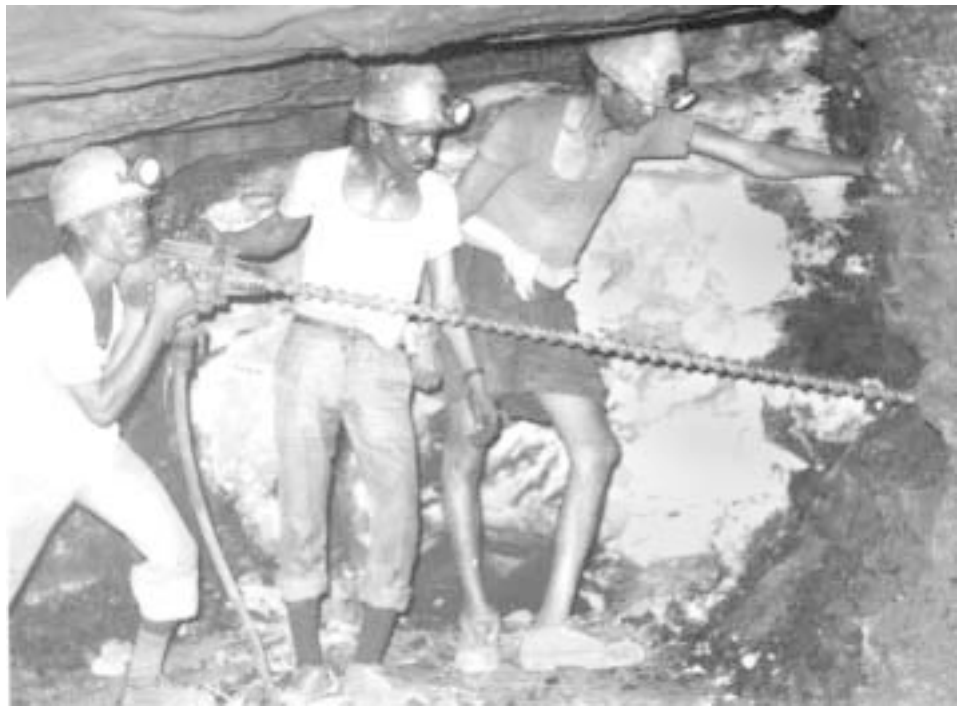
A long drill is used to make a hole for the dynamite
